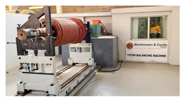
The comprehensive scope of work involved dismantling, cleaning, and assessing all parts of the motors. The team at then dynamically balanced the rotors at operating speed using their own 12-tonne balancing machine.
