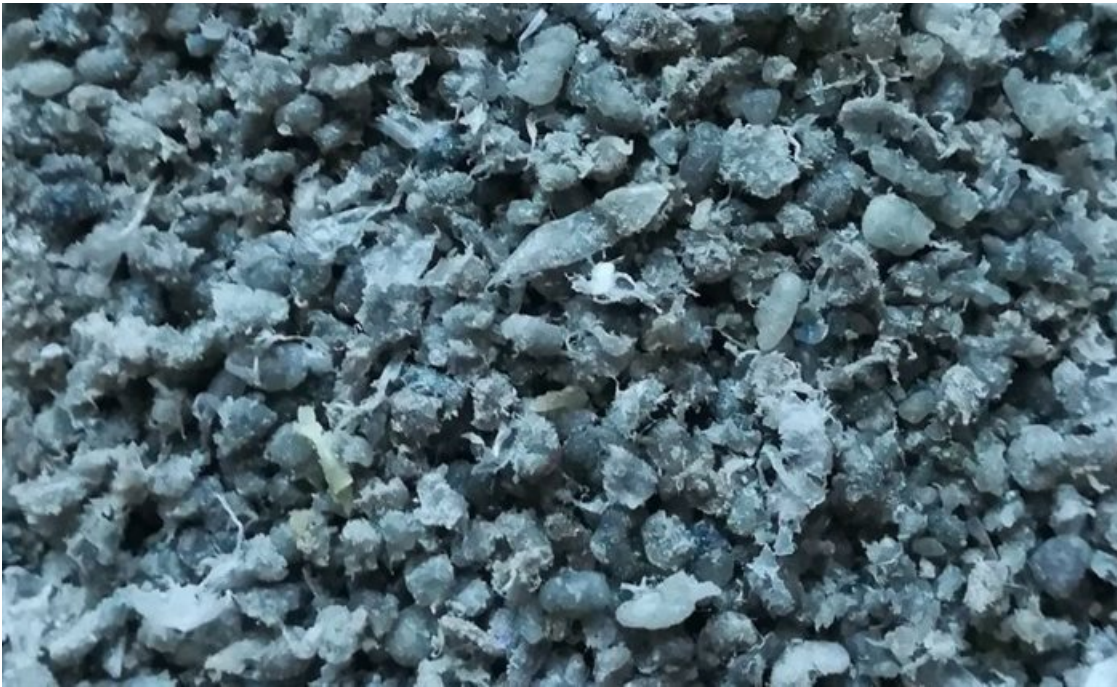
Dr Abubakar Sadiq Mohammed developed a wood-plastic composite using a mix of biomass from all parts of a Port Jackson tree ( Acacia saligna ) and recycled, low-density polyethylene. Source: Supplied
